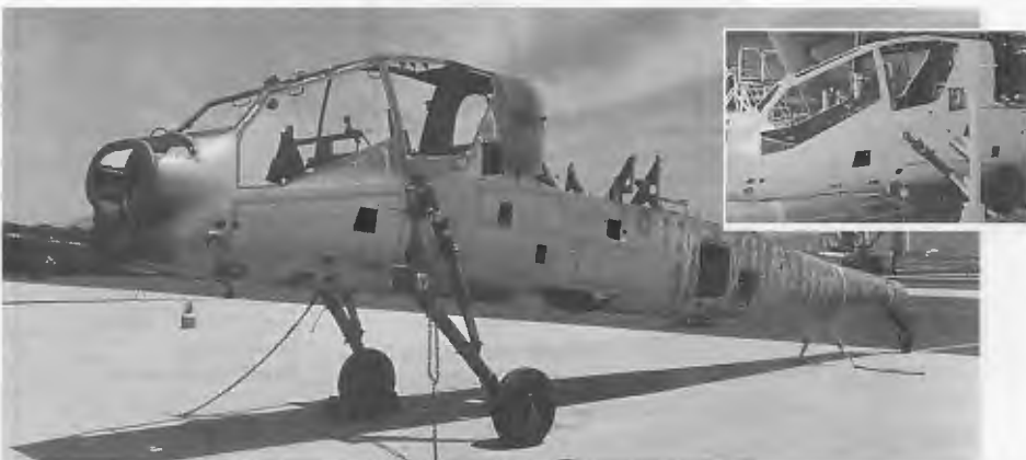
During the re-manufacturing process to become AH-64D Longbow Apaches, original AH-64s are stripped to the basic airframe and rebuilt from the guts out. Inset: stripped and re-primed, Apache begins the rebuild process.
